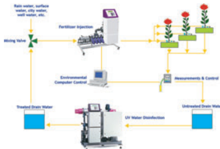
A closed recirculation system works by recycling water from the greenhouse and storing it in a covered holding tank.
