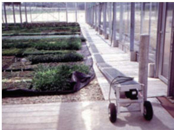
Top: Belt conveyors help speed the movement of transplanted containers from the headhouse to the growing area. Middle: A belt conveyor on wheels that can be moved into a trailer reduces considerable walking when loading or unloading. Bottom: This 80-ft. sectional belt conveyor is powered by a single electric motor. (All photos courtesy of John Bartok, Jr.)
