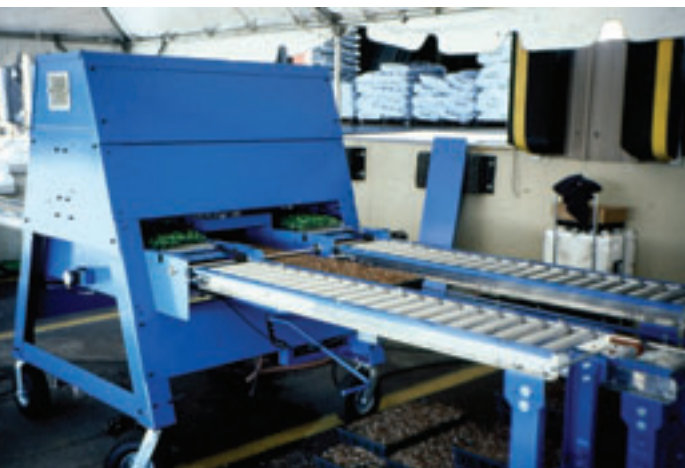
Left: Roller conveyors can be used to accumulate plants from a transplanter or transplanting conveyor prior to loading onto carts. Middle: Lightweight roller conveyors can be installed to hold plants for order picking. Conveyors are kept full by loading plants from the high end. Right: The low-cost trolley conveyor can move 10-30 flats at one time. Curved sections and switches allow movement between the headhouse and greenhouses.
