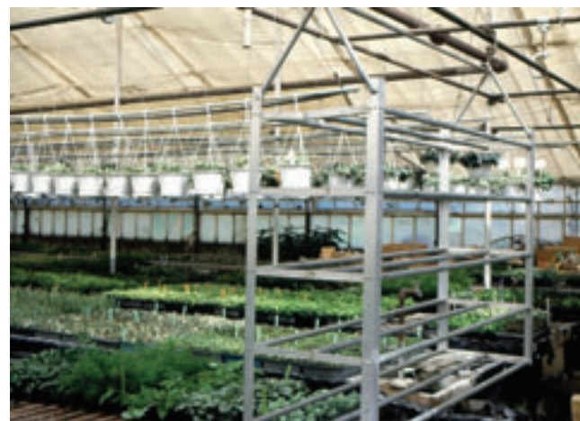
Left: Roller conveyors can be used to accumulate plants from a transplanter or transplanting conveyor prior to loading onto carts. Middle: Lightweight roller conveyors can be installed to hold plants for order picking. Conveyors are kept full by loading plants from the high end. Right: The low-cost trolley conveyor can move 10-30 flats at one time. Curved sections and switches allow movement between the headhouse and greenhouses.
