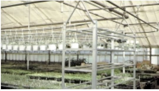
A trolley conveyor will move 20-40 flats at one time.
