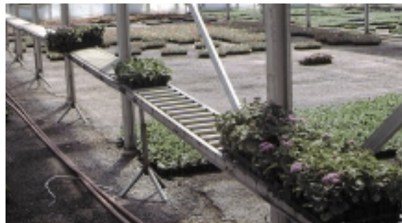
Low-cost roller conveyors have many applications in a greenhouse business.
