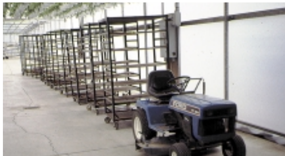
A tractor-pulled cart train speeds handling for distances over 200 feet.
