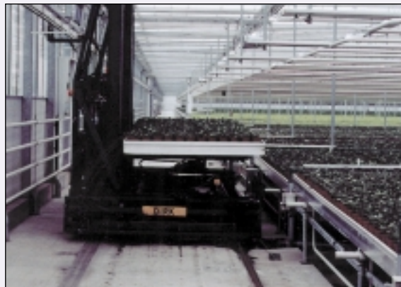
Automated benches can easily be moved from headhouse to production area with a simple manual cart (top) or an automated transport system (bottom).
