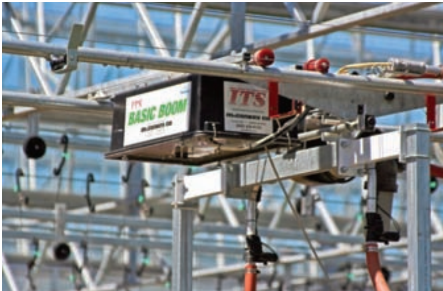
Booms can be remote started, programmed or monitored by PC, in addition to direct controls. They can be operated from a Sensaphone or Blackberry, in some cases.
