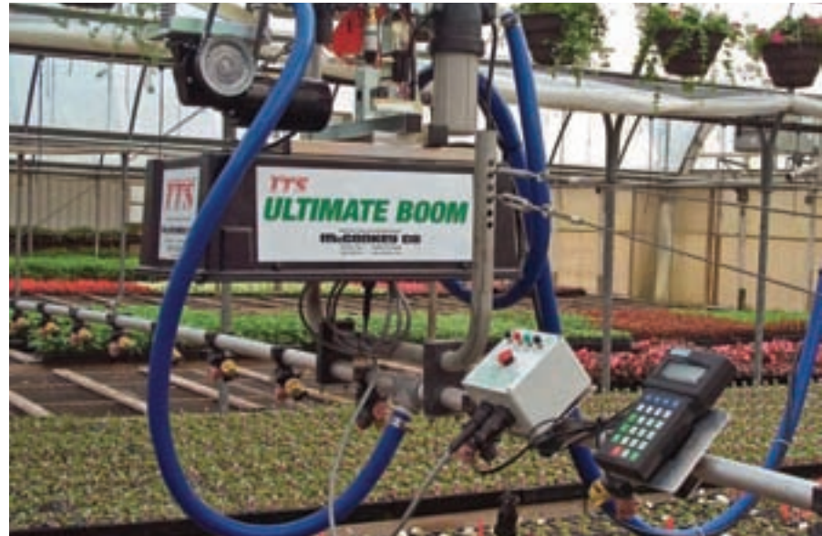
Booms can be remote started, programmed or monitored by PC, in addition to direct controls. They can be operated from a Sensaphone or Blackberry, in some cases.
