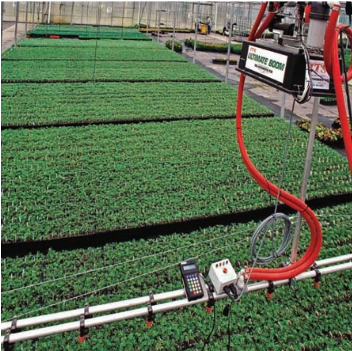
Spray bars on boom irrigation systems can span the entire width of the greenhouse.
