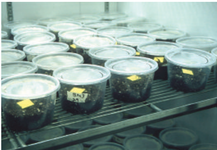
Deli containers with growing media containing diatomaceous earth inside an environmental control chamber. A yellow sticky card was placed on the surface to capture adult fungus gnats that emerged. (Photos courtesy of Ray Cloyd)
