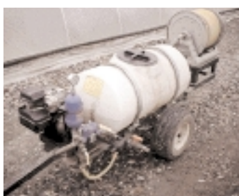
Top: Gas engine-powered hydraulic sprayer with cart. Middle: Hydraulic rechargeable backpack sprayer. Bottom: Gas engine-powered hydraulic sprayer with hose reel and spray gun. (All photos courtesy of John Bartok)
