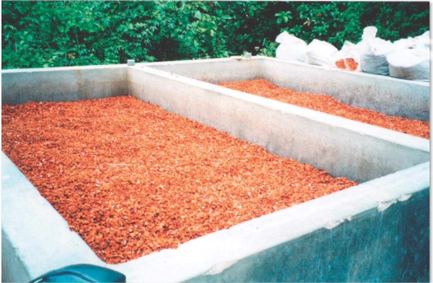
Coir washing bins. (Photos courtesy of Millenniumsoils Coir)
