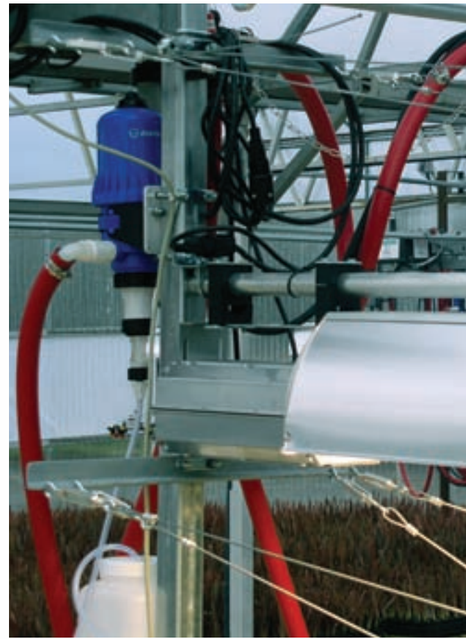
Boom systems can provide versatility to a greenhouse by performing additional tasks such as lighting. (Photo: Solaris, a Division of McConkey Co.)
