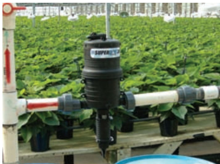
By using a formula, you can determine the amount of fertilizer needed to inject into irrigation water. (Photo: Dosmatic USA/International, Inc.)
