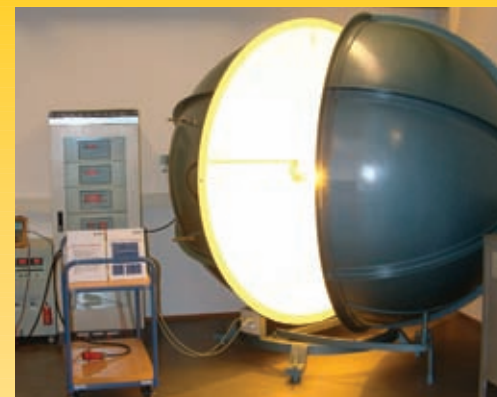
The Ulbrich Sphere can test the lumen/PAR light output of any bulb.
