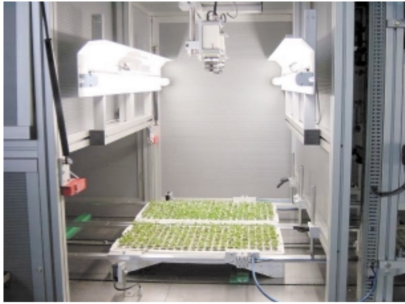
During the first phase of replugging, a camera records which cells need to be replaced and transfers that information to the equipment that actually does the plugging. (Photos courtesy of Nexus Corporation)
