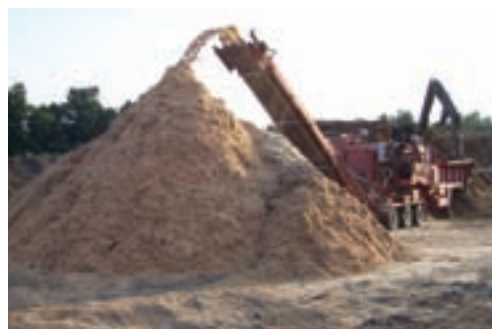
Pine tree substrates can be produced from freshly harvested pine trees — Loblolly pine has been researched the most, but eastern white pine shows promise — that are chipped and ground in a hammer mill.
