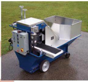
This trayfiller is easy to adjust and flexible to different tray sizes. Its best element is its quality of filling.
