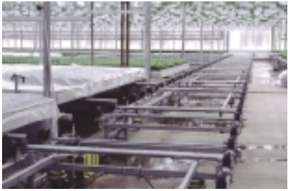
Bench-moving rails for the movable tray system.
