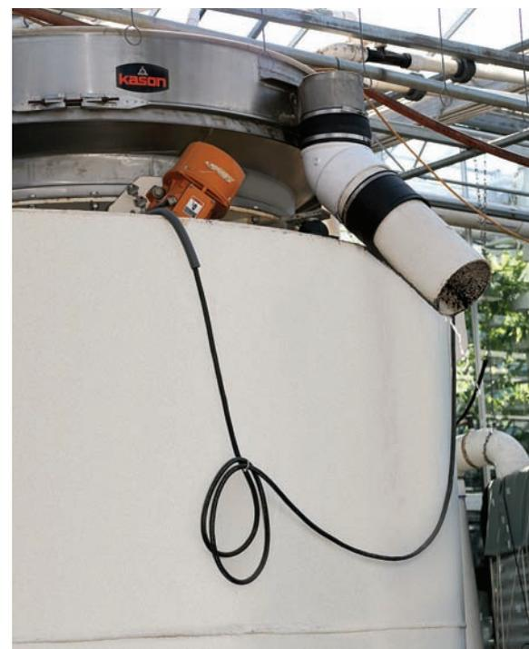
Greenhouse water flows through the screener into a 10,000-gal. main storage tank while debris falls into a tote.
