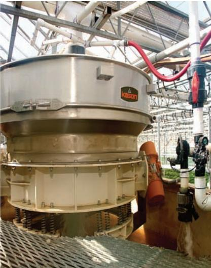
The 72-inch-diameter Kason Flo-Thru Vibroscreen separator screens up to 500,000 gals. of water per day. Side-mounted motors reduce height of the screener, allowing it to fit between the ceiling and top of the storage tank.
