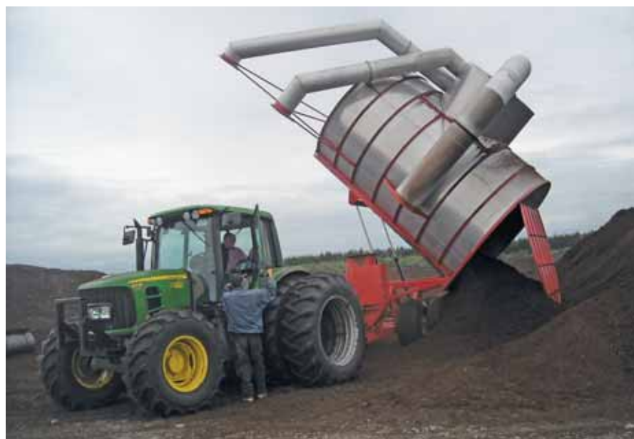
Figure 4. The contents of a vacuum harvester are emptied.
