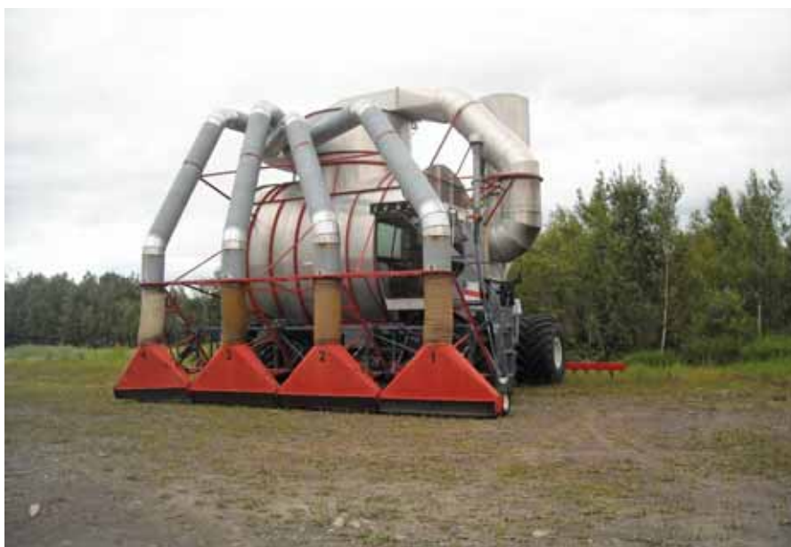
Figure 3. A large “four-headed” vacuum harvester.
