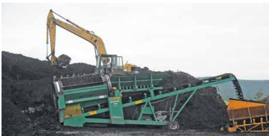
Figure 5. Peat is loaded onto a conveyer line for screening.
