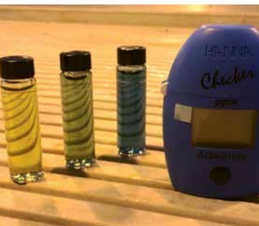
Figure 1. Alkalinity meters make it easy to check your carrier water alkalinity in house.
