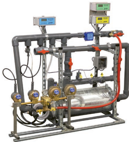
Injectors mix highly concentrated stock solutions with water at a specific ratio. (Photo: HE Anderson)
