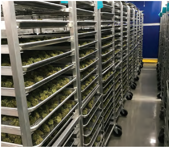
Cannabis growers who handle large quantities of buds can use rolling racks equipped with perforated trays that are easily moved into environmentally controlled drying rooms. (Photo: Fred Green, Fred Green Consulting)
