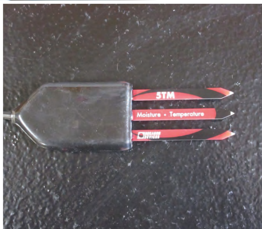
Figure 2a. The Meter Group makes this moisture sensor, the 5TM. It monitors soil moisture and temperature. This sensor is approximately 2 inches long, so it will fit in a 4-inch pot.
