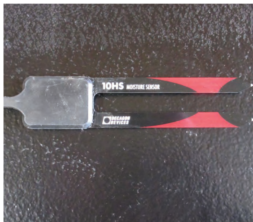
Figure 2b. The 10HS sensor is also made by the Meter Group. It only measures soil moisture, but it is larger than the 5TM sensor (approximately 4 to 5 inches long). It may be a good choice for perennial production in larger containers.
