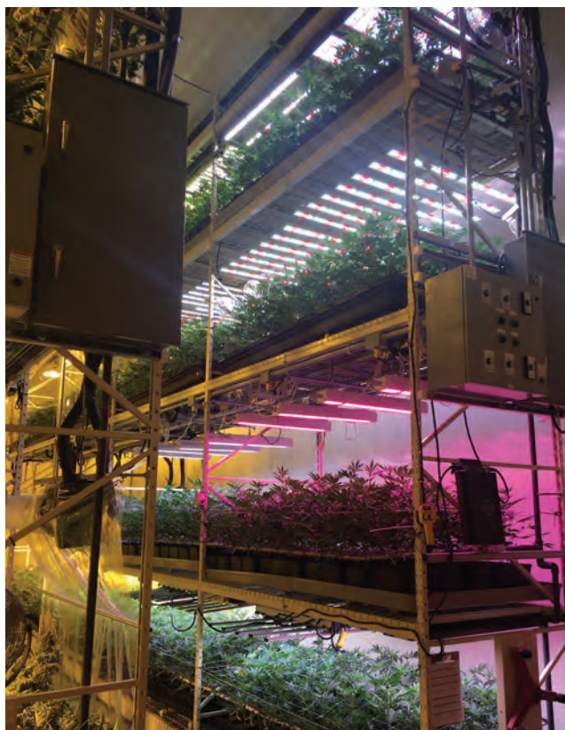
Using high plant density production can increase productivity and number of tiers; here Greenseal was performing an experimental lighting design.
