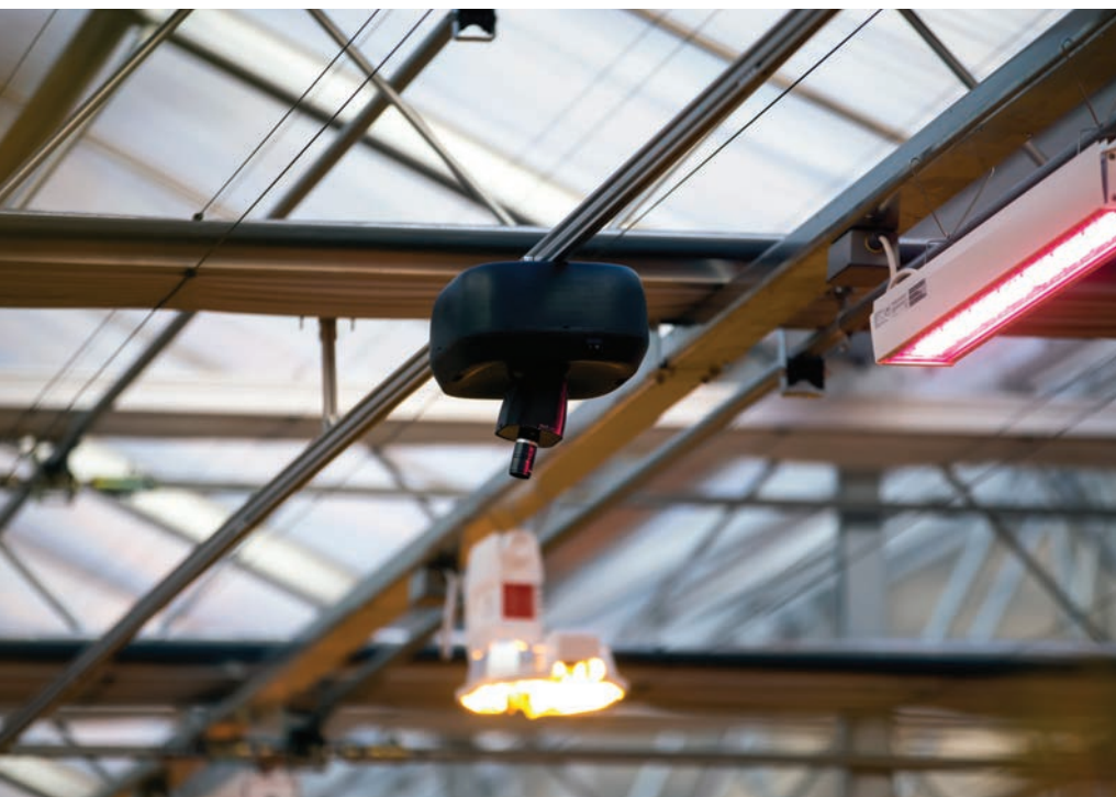
iUNU's AI system, called LUNA, incorporates video cameras that travel through a production facility on rails.
