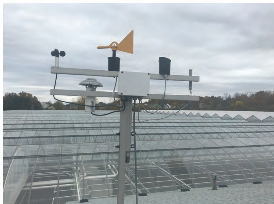
Figure 1. A pyranometer mounted on a weather station atop a greenhouse. (Photo: Jonah Brown)
