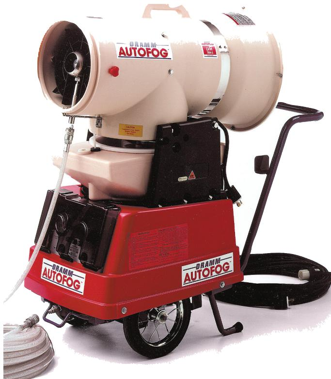
**Top:** Low-volume foggers use less water or carriers to apply insecticides, fungicides, disinfectants and fertilizers to greenhouse crops. **Bottom:** By creating billions of tiny spray droplets, ultra-low volume systems can treat large areas with less chemical solution. (Photos: Damm Corporation)
